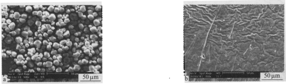
Fig. 1 SEM micrograph of native cornstarch granules(a) and the fracture face of FPTPS(b)
